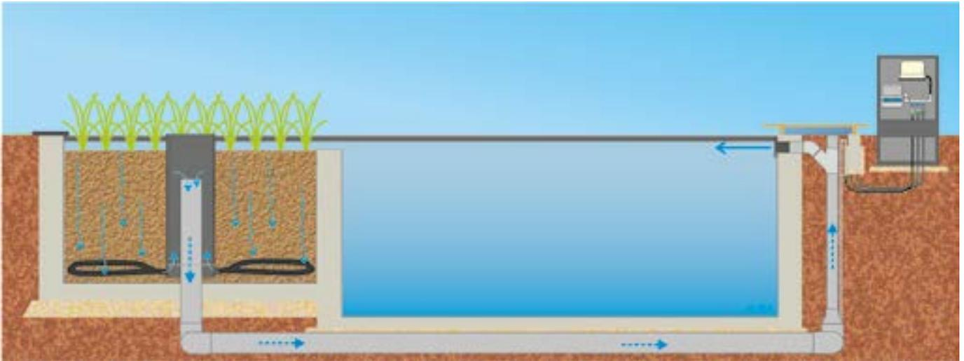
Pumps are always needed to continually circulate (swimming) pond water through a biological filter.
