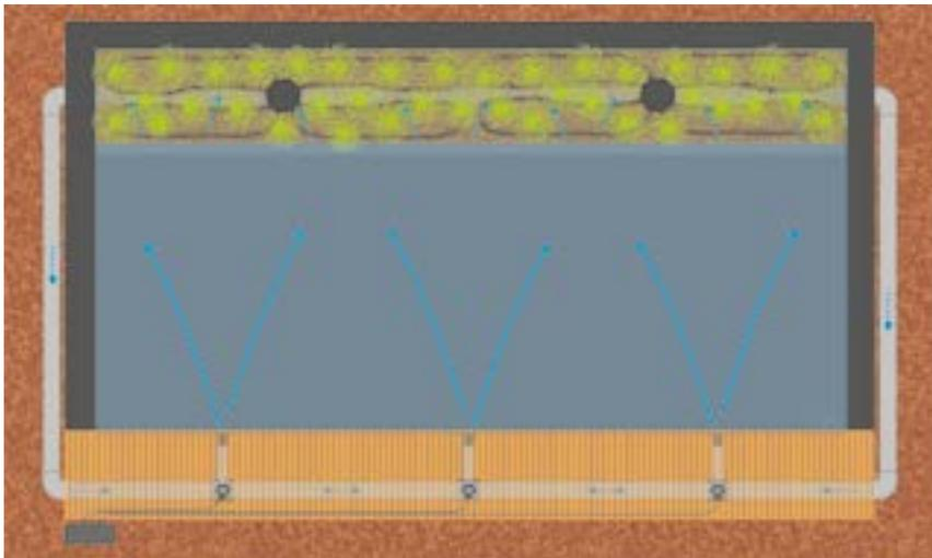
The illustration shows how 3 Airlift pipes circulate the water in a down-flow swimming pond. 3 Airlift pipes in combination with a 67 W NITTO air pump transport about 20 m<sup>3</sup> water per hour.
