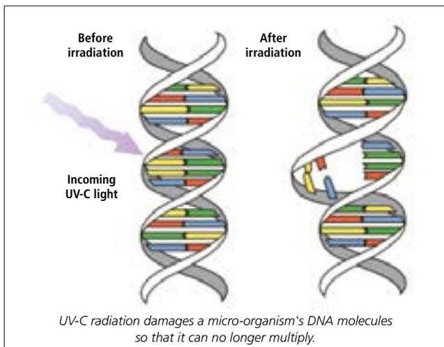
UV-C is electromagnetic radiation, which penetrates the cell wall of micro-organisms and damages their nucleus. This destroys their ability to multiply, so they die and have to be filtered out of the water.
