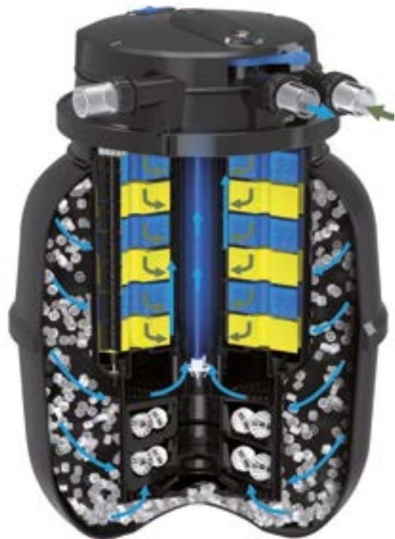
Pond water is pumped through the filter foam pack to the BioCell or BioBall pack. The cleaned water then flows past the UV-C clarifier for elimination of floating algae. The water then flows back to the pond.
