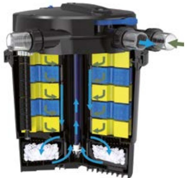
Pond water is pumped through the filter foam pack to the BioCell or BioBall pack. The cleaned water then flows past the UV-C clarifier for elimination of floating algae. The water then flows back to the pond.
